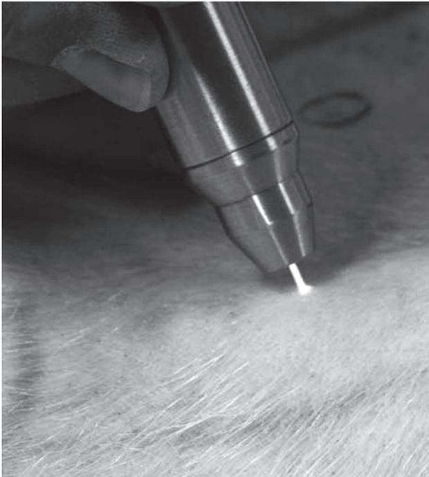
**Figure 1** Plasma-jet under working conditions
